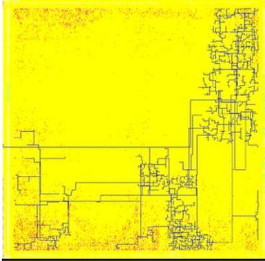
Fig. 14 Clock tree in silicon level.
