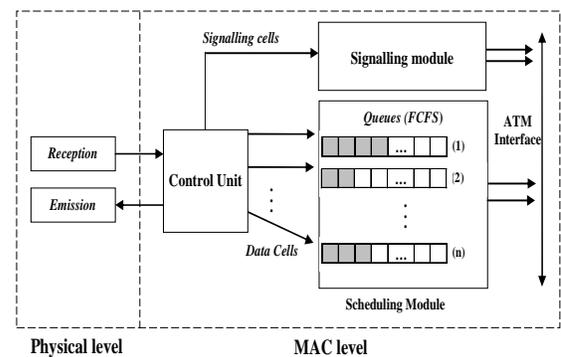
Fig. 3 AP radio medium architecture in WATM.
