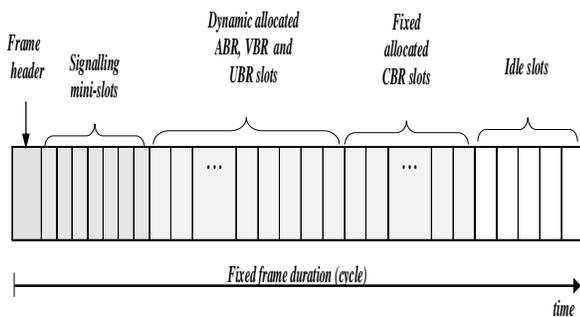
Fig. 1 Dynamic TDMAUPLINK access control frame format.
