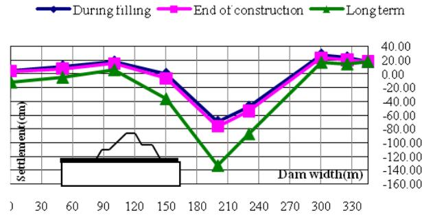
Fig. (4). Settlement at the interface embankment-foundation- Drucker-Prager model
