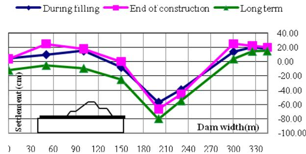
Fig. (3). Settlement at the interface embankment-foundation-Elastic model
