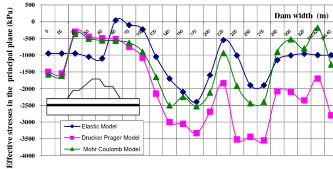
Fig. (14). Effective stress calculated in the principal plane at the middle of the dam foundation by different behaviour models at long term.
