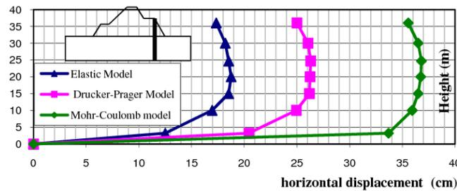
Fig. (9). Horizontal displacement of the downstream shoulder at the end of construction.
